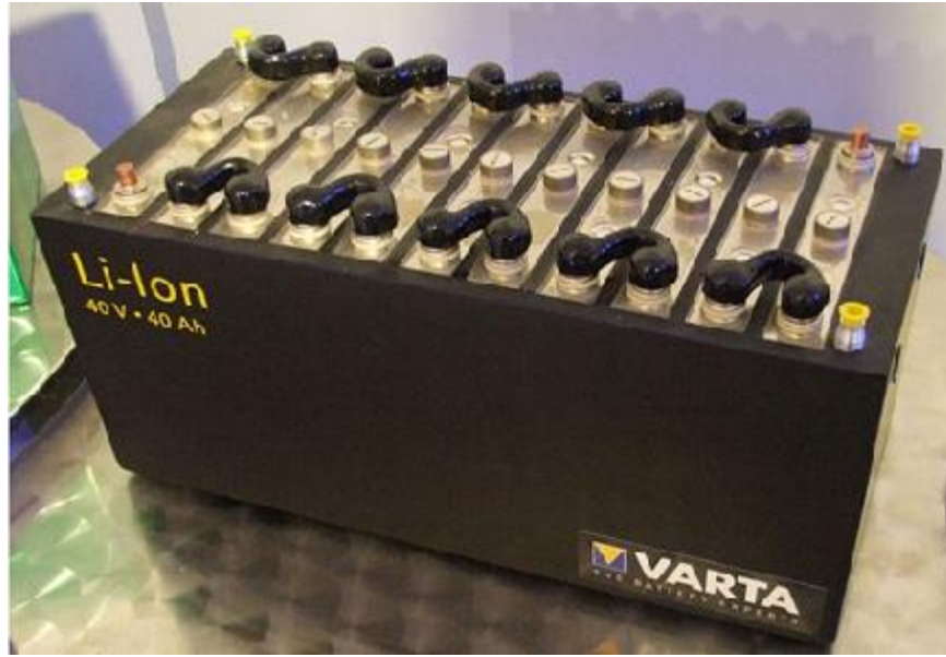
Figure 3.1. Typical initial Lithium ion battery pack
